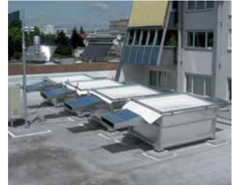
Hotboxes for the measurement of thermal behaviour of multilayer membrane assemblies
