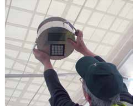
Measurement of membrane stresses on site
